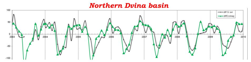
Basin TWS (= sum of all surface water, soil moisture, snow water, and groundwater) is simulated by ECOMAG with daily time step
