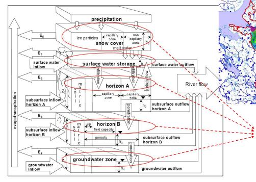
Basin TWS (= sum of all surface water, soil moisture, snow water, and groundwater) is simulated by ECOMAG with daily time step
